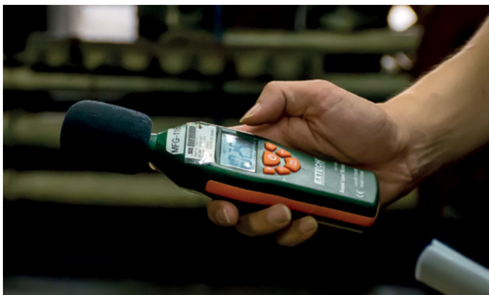
Checking sound levels
